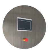
Fully automated control with Allen Bradley HMI & PLC
